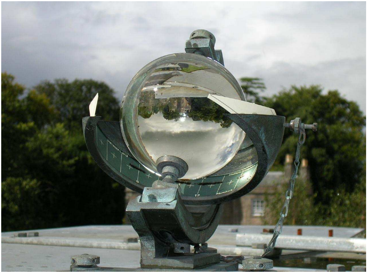
Plate 1. The Campbell-Stokes Sunshine Recorder in Aug 2005 (photo - CJB)
