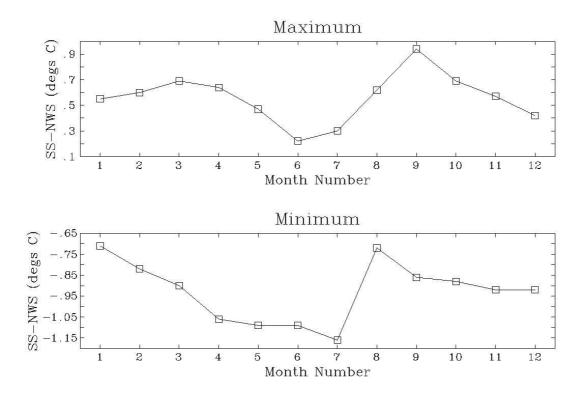
Figure 2: The difference between the mean monthly temperature extrema measured by the Self-Recording Thermograph in a north-wall screen and the standard maximum and minimum thermometers in a Stevenson Screen at Valentia Observatory from 1955 to 1959.
