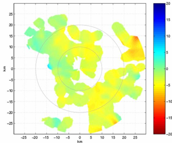
**Figure 3. Refractivity change between 03:00 and 04:00, 30/09/2007 from the Cobbacombe Cross radar. A refractivity unit (N) is approximately equal to a 1% change in relative humidity (courtesy J. Nichol).**
