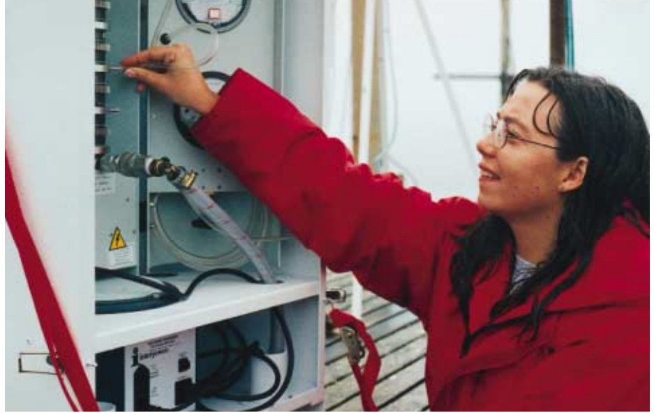
Rebecca Webb, from the University of Tasmania, adjusts the aerosol sampler flow rate on the roof of the Cape Grim station.
