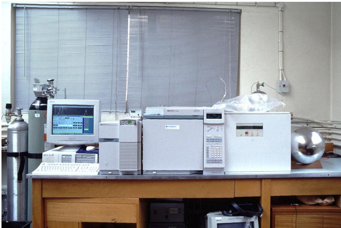
**Figure 3.1:** Analytical System, ADS-GC-NICI-MS.
