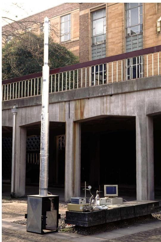
**Figure 2.1:** Tracer Release Apparatus.
