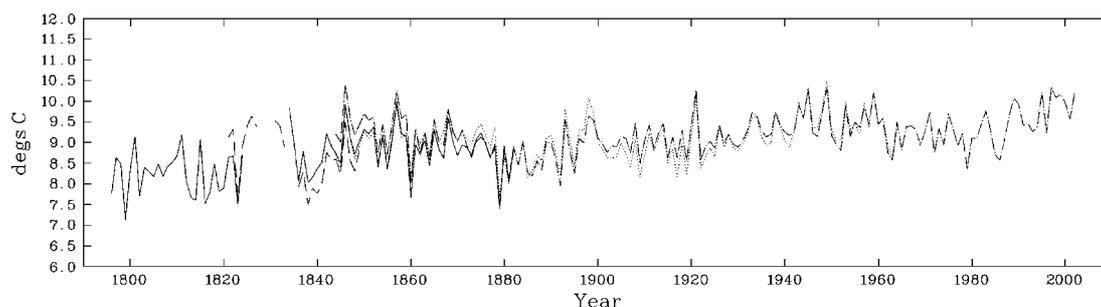
Figure 6. Mean annual temperatures at Armagh Observatory 1796–2002 from three independent sets of observations. Series I (continuous line), Series II (dashed–dotted line) and Series III (dotted line) and the Dunsink patch (dashed line)
